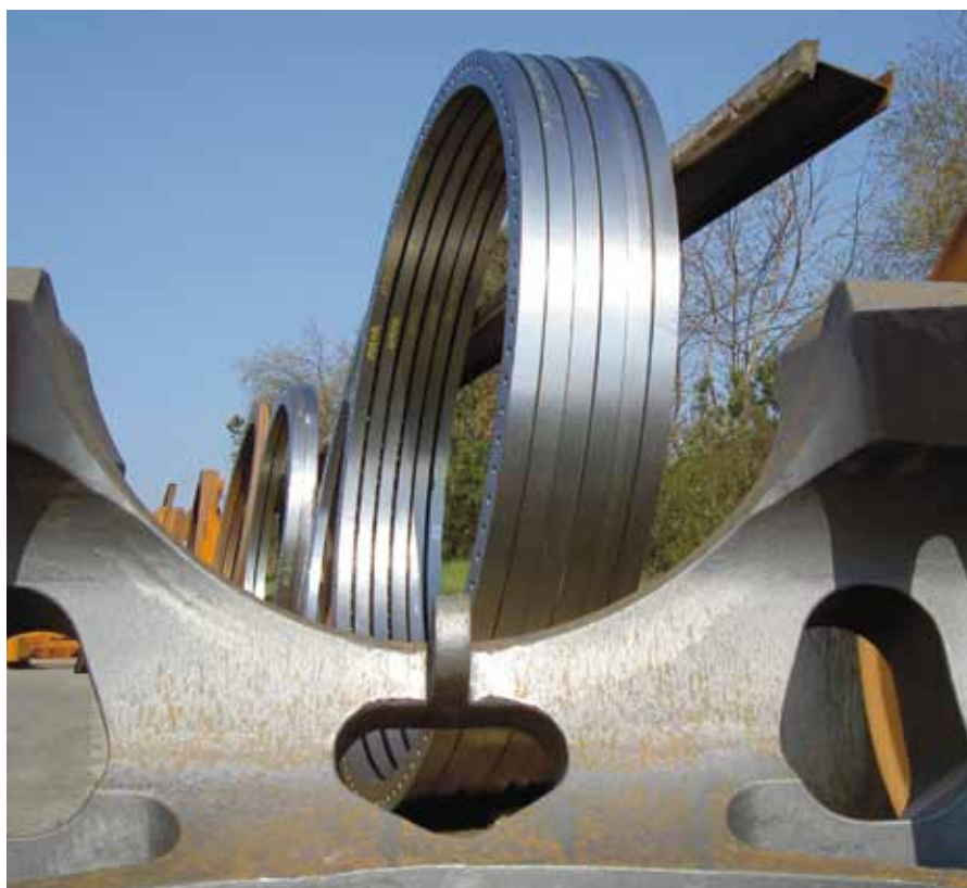
Flanges are used to attach the tower components in a wind turbine. The flanges can be up to 8 metres in diameter and weigh as much as 15 tonnes.
